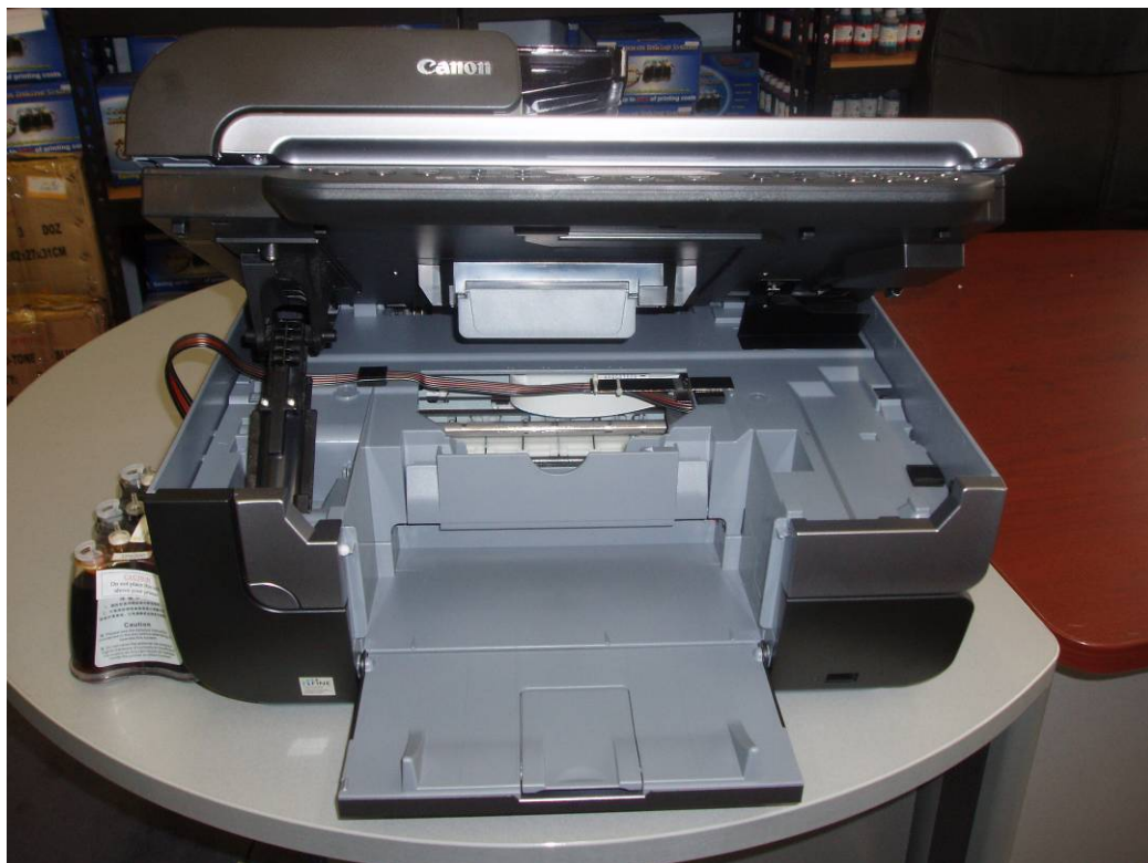
Installed CISS system on a Canon MP530 series printer
